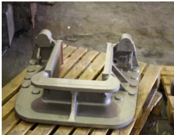
Casting of horn block
